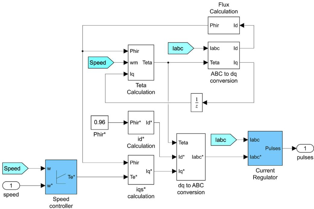
Fig. 2 Cascade Speed, current control system of AGV drive.
