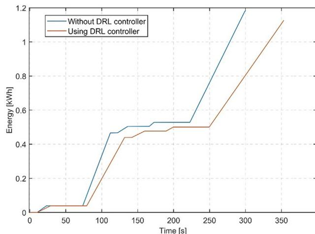
**Fig. 9** AGV energy consumption comparison without DRL controller and using DRL controller agent.
