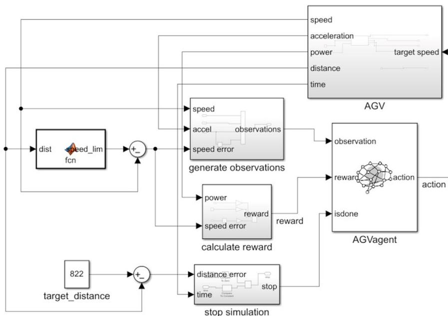
Fig. 6 Simulink model of deep reinforcement learning-based AGV control for container transportation.
