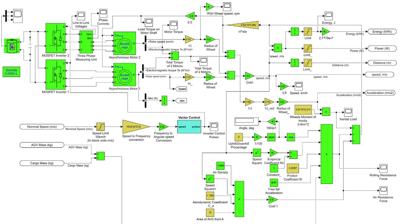
Fig. 3 AGV drive system Simulink model.
