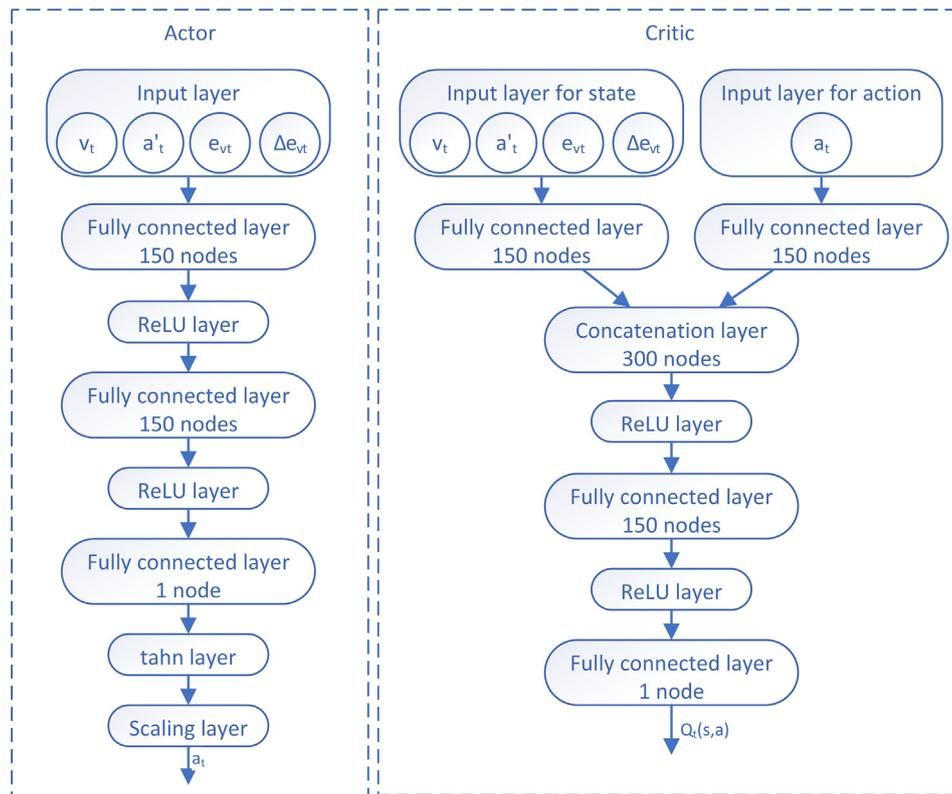
Fig. 4 Deep neural network architectures for actor and critic.
